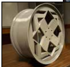
Advanced CAD student Dalton Wells designed his own custom rim which was 3D printed. The print job took about 90 hours to complete.
